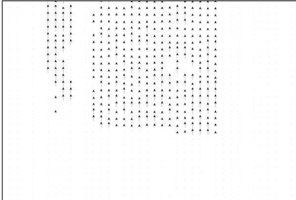
Figure 7: Reactions proposed by active cells at frame  $ta$ . Robot is far from the door and cells propose to go straight on.
