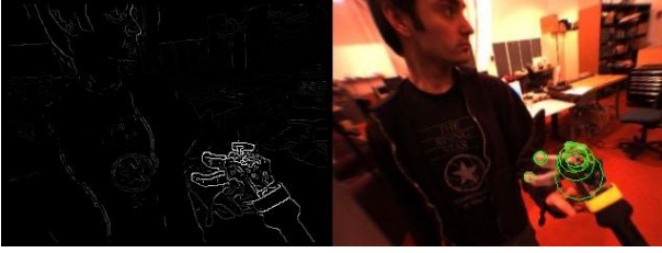
Figure 4: A sample output of the visual attention system selecting salient image regions during hand-discovery. The input is 120 \times 160 image frames captured at 20 – 30 fps in an everyday, cluttered environment (right). The visual attention system prefers rapidly moving shapes that are approximately convex. The edge motion is measured relative to the global image motion (left). Image patches are selected from the top 10 regions (the circles around the robot’s hand).
