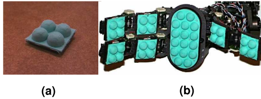
Figure 2: Obrero’s hand and detail of the tactile sensors. (a) Group of four tactile sensors. The deformation of each of them is measured by a total of four sensors. (b) Tactile sensors mounted on the hand.
