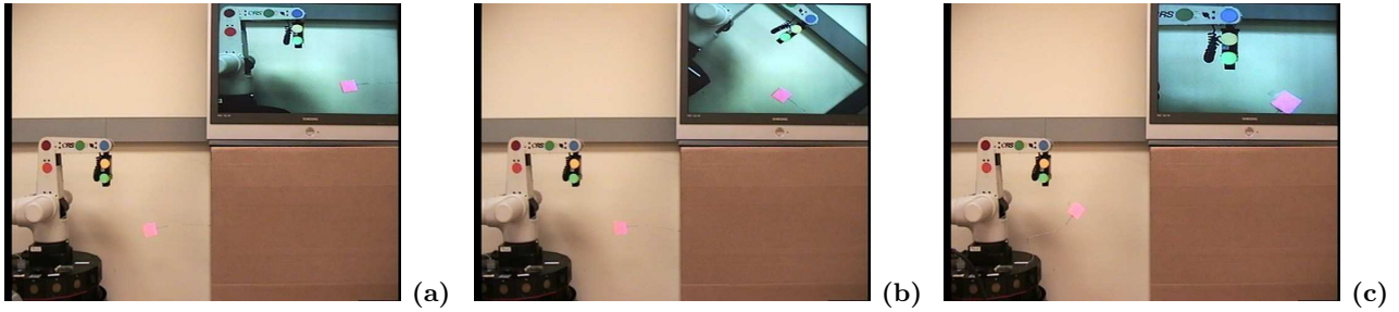
Figure 10: The figure shows three views from the robot's camera, one for each of the three experimental conditions. The image of the robot in the TV is: a) approximately the same size as the real robot; b) rotated by negative 50^\circ ; and c) scaled (zoomed in) by a factor of 1.6. During the video-guided grasping experiments, however, the robot cannot observe its own body (see Figure 3.b)
