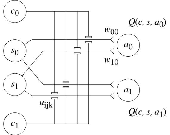
Figure 2: The approximation of  $Q(c, s, a_j)$  as an artificial neural network with shunting inhibition from the context nodes  $c_k$  to the association between a state node  $s_i$  and an action node  $a_j$ .
