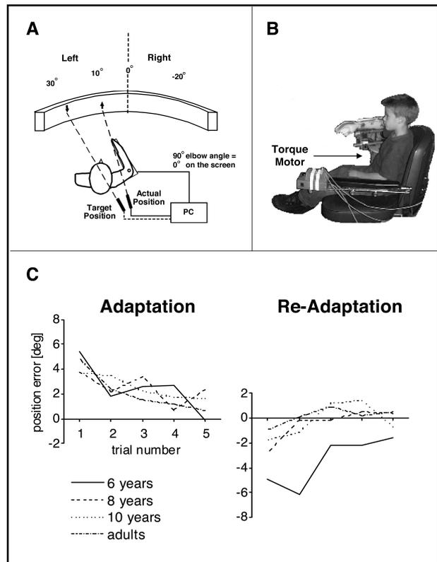
Figure 2: Development of force adaptation. **A.** Subjects performed goal-directed forearm movements against an assisting viscous force. **B.** The viscous force was provided by a computer-controlled torque motor. **C.** Adaptation rates were similar in all age groups, but re-adaptation was less complete in the 6-year-old children. Shown is here the positional error at the end of the first movement unit. Modified from: Jansen-Osmann et al. (2002)
