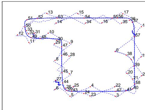
FIG. 2 – Simulation of the place-action learning during a path-learning session. The figure shows the trajectory during the learning (clockwise travel). Numbers correspond to the position and the order of the places autonomously learned by the robot. The professor first forbids the robot to escape from the path (two laps of proscriptive learning), and then guides the robot on the precise trajectory (several laps of prescriptive learning). The number of learned places stops increasing quickly.
