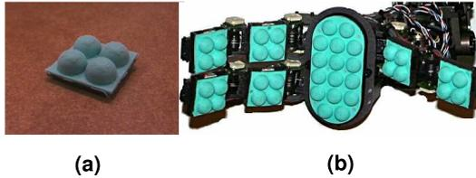
Figure 2: Obrero’s hand and detail of the tactile sensors. (a) Group of four tactile sensors. The deformation of each of them is measured by a total of four sensors. (b) Tactile sensors mounted on the hand.
