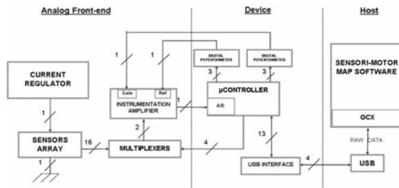
Figure 4 – Block schema of the acquisition hardware
