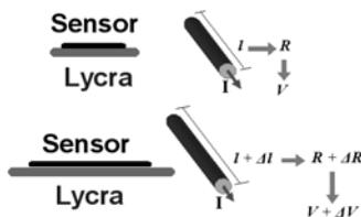
Figure 3 – Transduction principle of the strain sensor
