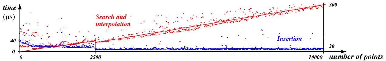
Figure 8: The computation performance for the access and insertion of a single point in the BSP tree is shown in blue. The interpolation process (finding the leaves and iterating on the points properties) is displayed in red. Both are expressed in  $\mu s$  and depend on the number of points present in the tree structure. Of course the points repartition in the state space has a great influence but the tree rapidly becomes locally balanced.
