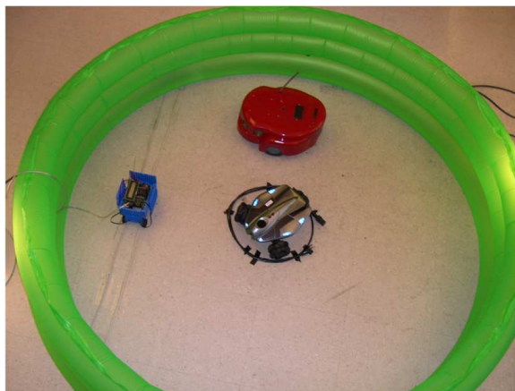
Figure 1: The experimental environment with the developing Rovio robot in the center, a larger static red robot, and a smaller moving blue robot.
