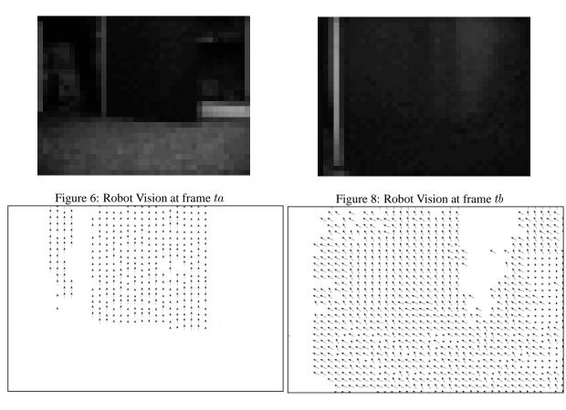
Figure 7: Reactions proposed by active cells at frame ta. Robot is far from the door and cells propose to go straight on.
