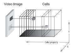
Figure 2: Cells data structure used to capture a behavior. The fourth dimension (neighborhood density) is not shown.
