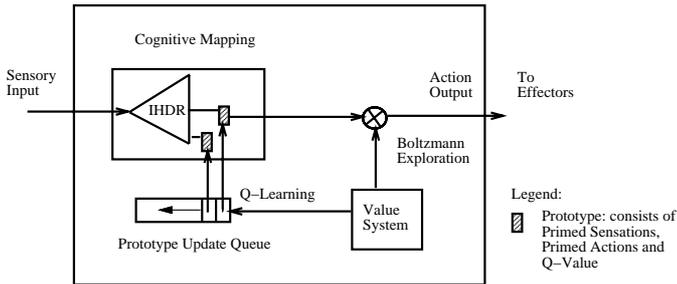
Figure 1: System architecture of SAIL experiments.
