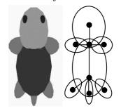
Figure 4: Kinematic structure of a simplified CG model with a fixed pelvis and 7 free joints. Total DoF is 14.
