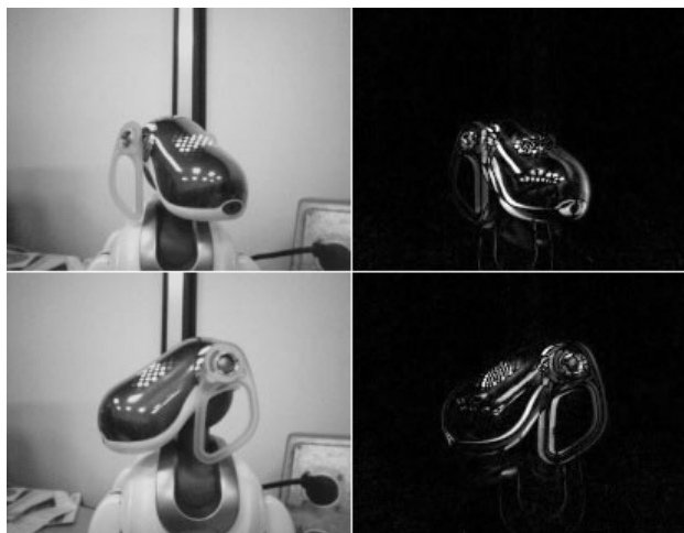
Figure 1: Detecting a robot's head orientation using slight movements around a central position.
