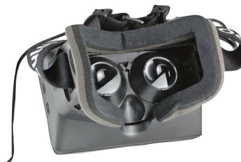
Figure 2. Back view of the Oculus Rift, the two eye screens can be seen (Figure reference: http://en.wikipedia.org/wiki/Oculus_Rift )
