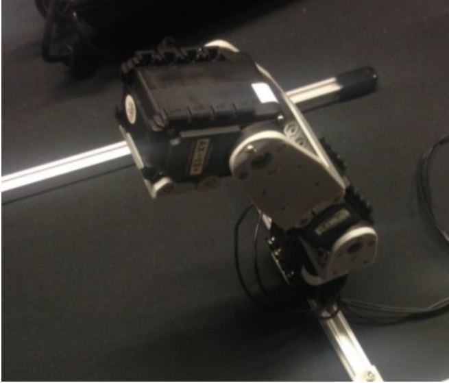
Figure 1: Robot arm with servo 1 at bottom, servo 2 in the middle, and servo 3 at the top
