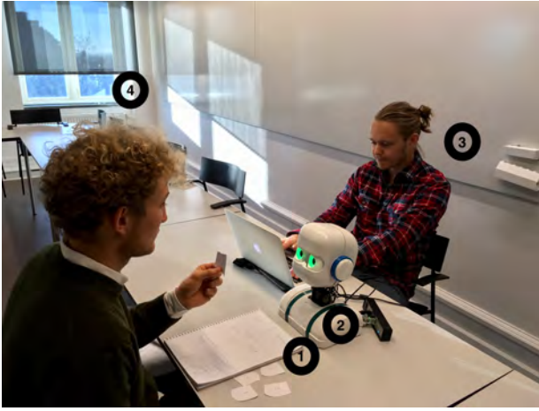
Figure 13 – Experiment setup for the final test. 1: Paper used to map mental states to robot behavior. Small pieces of paper were shown, and then placed on the large paper to indicate which mental state the robot had displayed. 2: The robot. 3: Experimental supervisor. 4: Participant.
