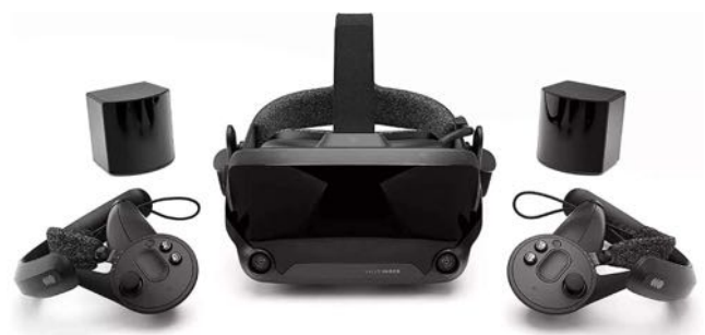
Figure 2. The Valve Index HMD virtual reality headset (middle), cameras (mid-left, mid-right), and controllers (far left, far right)
