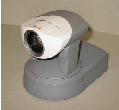
FIG. 3: An Axis 2130 PTZ is used in the robot setup. The camera has a built in web server which sends requested images in different resolution and compression
